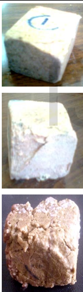
Fig. 10. Effects of sodium sulphate crystallization with white spotted sandstone. top)- after one cycle, middle)- after five cycles and bottom)- after 10 cycles.
