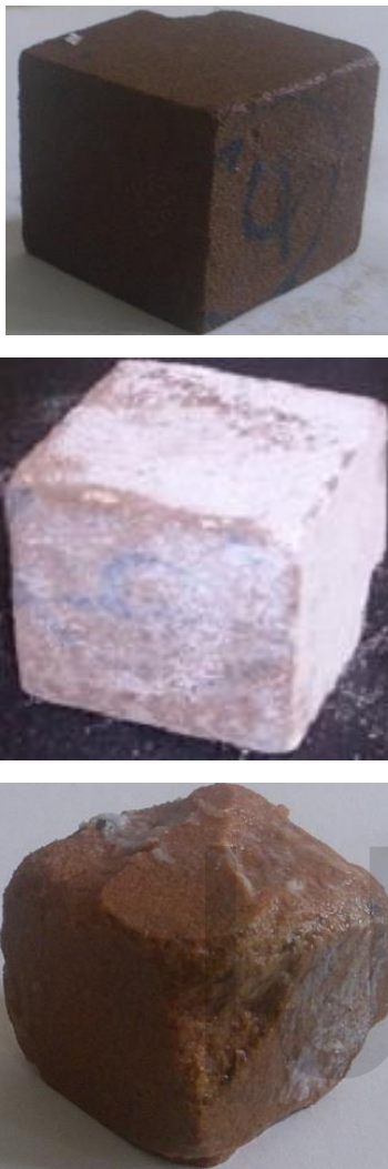
Fig. 11. Effects of sodium sulphate crystallization with reddish spotted sandstone.top)- after one cycle, middle)- after five cycles and bottom)- after 10 cycles.
